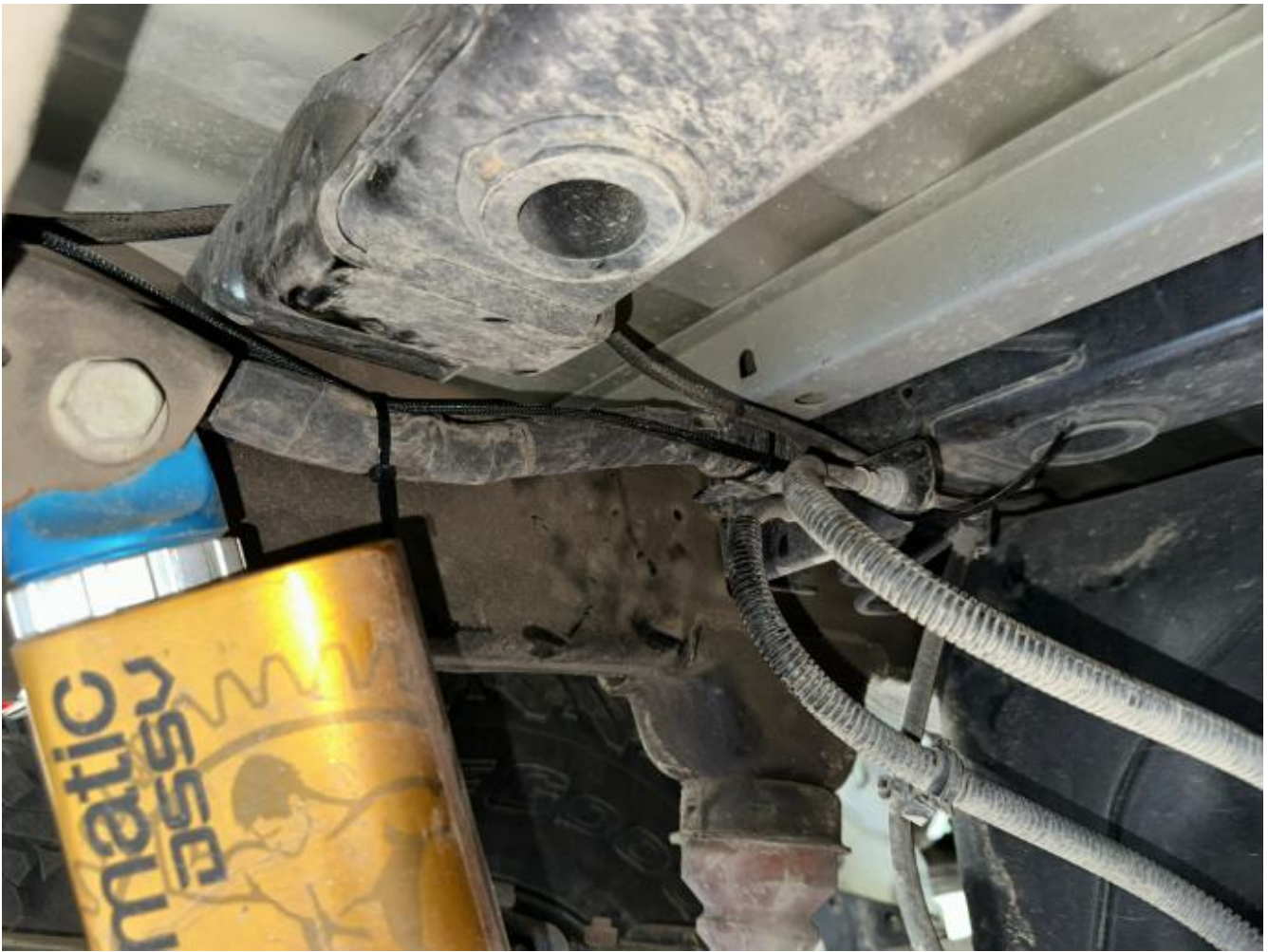
Additional image showing secures along the inboard side of the driver side frame rail.
