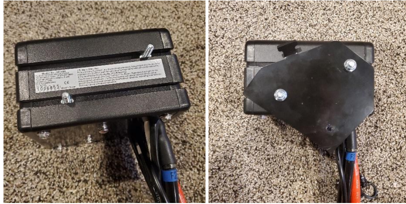
Bolt locations in controller t-slot for backplate
