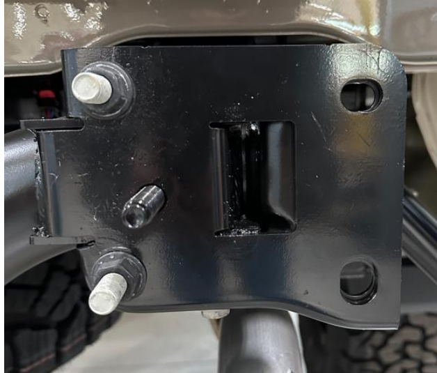
Photo 16: Hitch bracket installation
