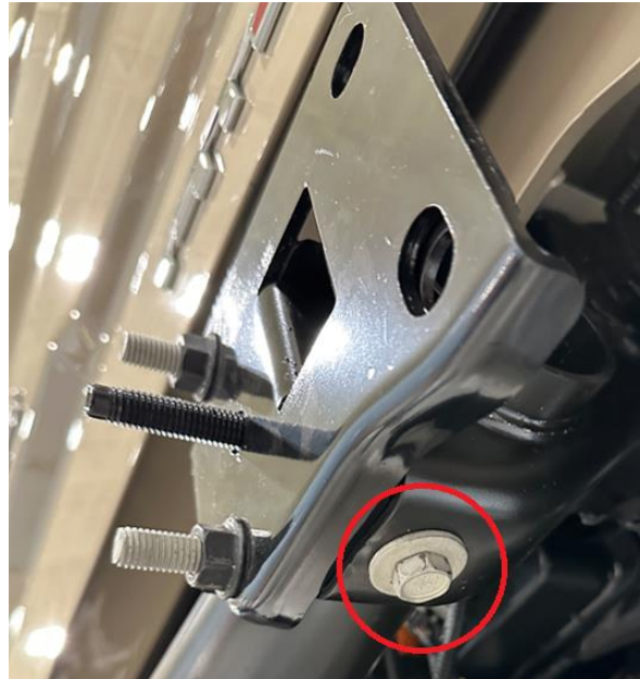
Photo 17: M10 bolt into bottom of hitch bracket
