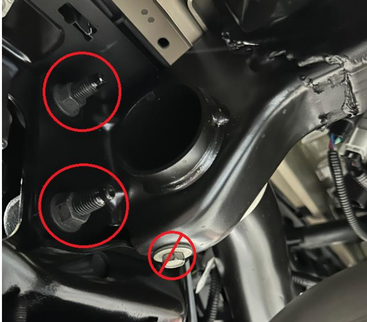
Photo 8: M12 nuts securing bumper
