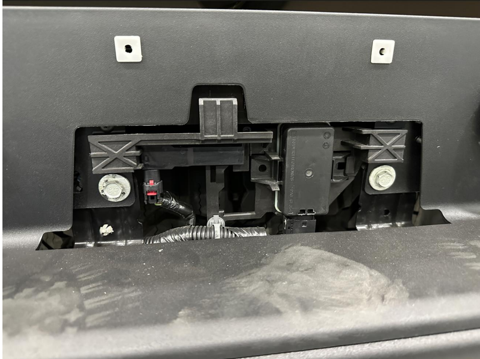
Photo 2: Passive entry sensor behind license plate
