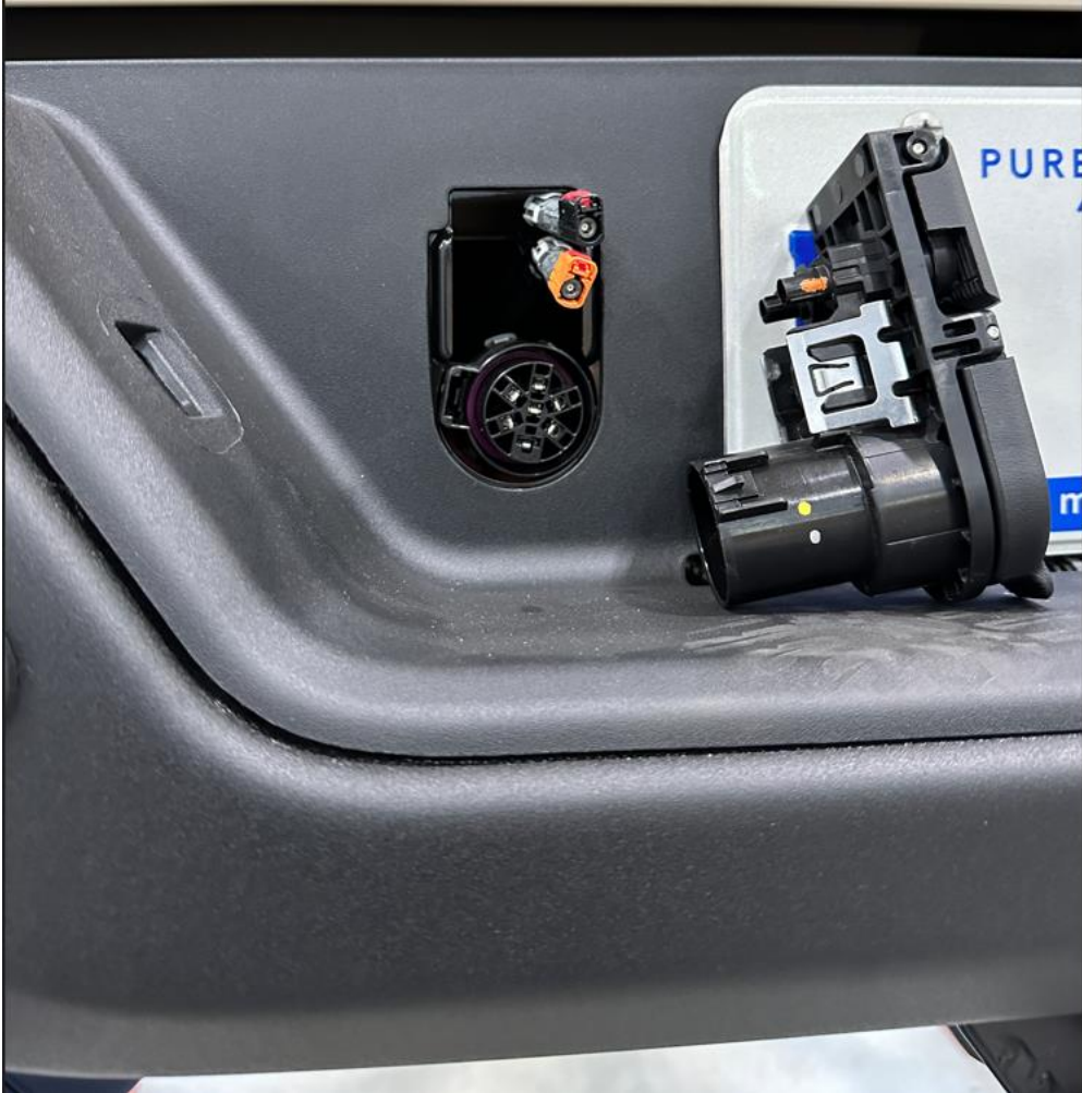
Photo 1: Removal of trailer plug
