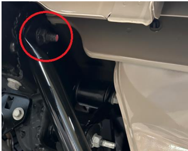
Photo 9: Upper pencil brace mounting location
