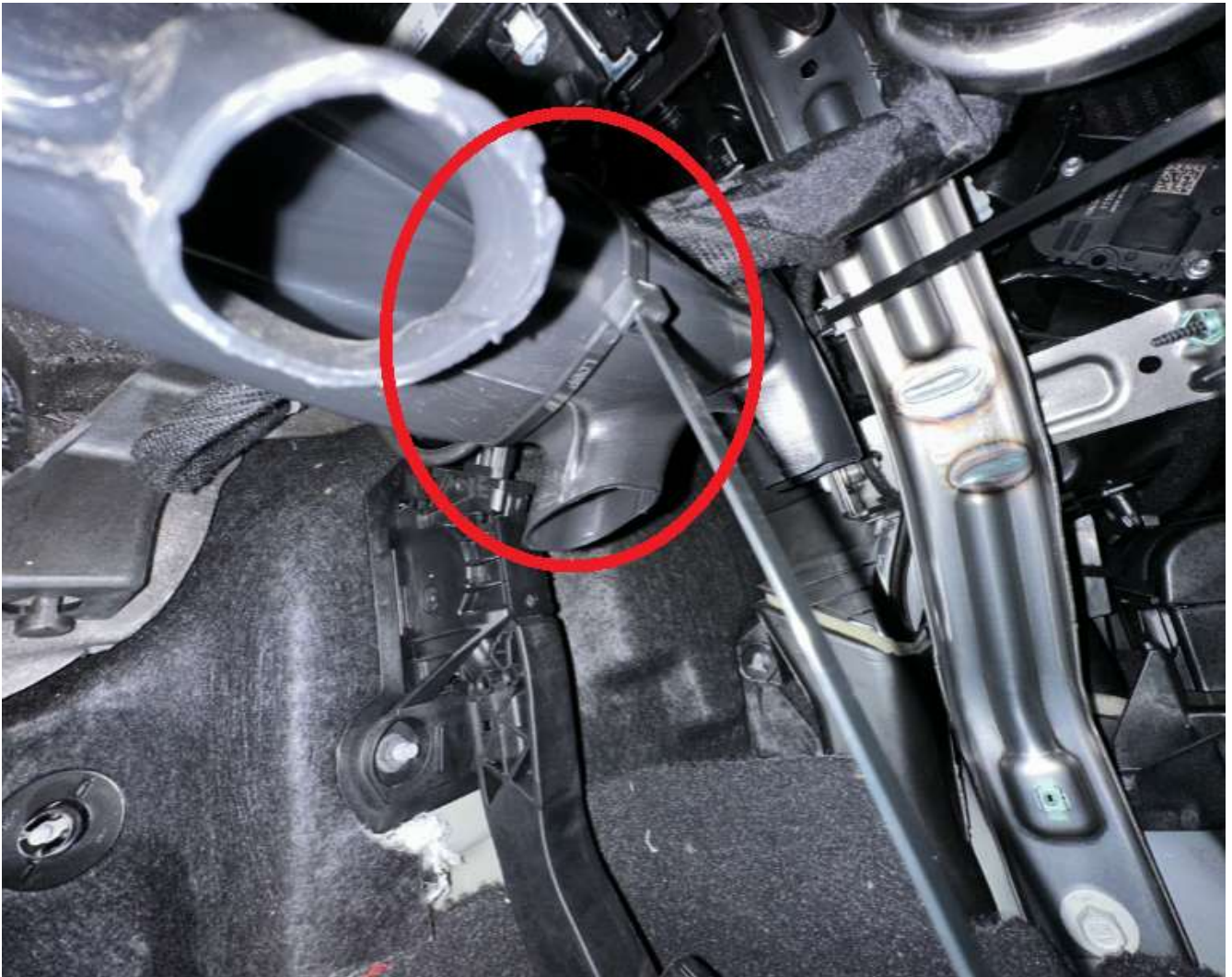
14. Staying on the drivers side, secure the harness to the AC vent as shown above.
