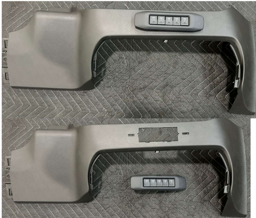
7. If installing aux switches, snap them into the new bezel. You can now begin installing the harness
