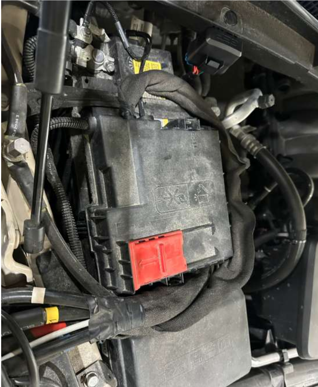
19. In the engine bay, remove the fuse box cover
