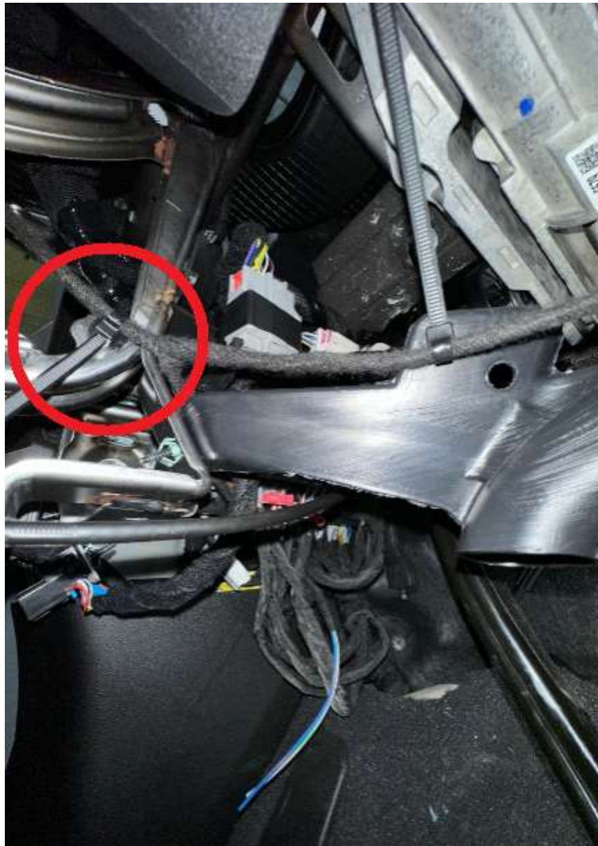
16. Using another fir tree zip tie, secure the harness to the metal bracket as shown.
