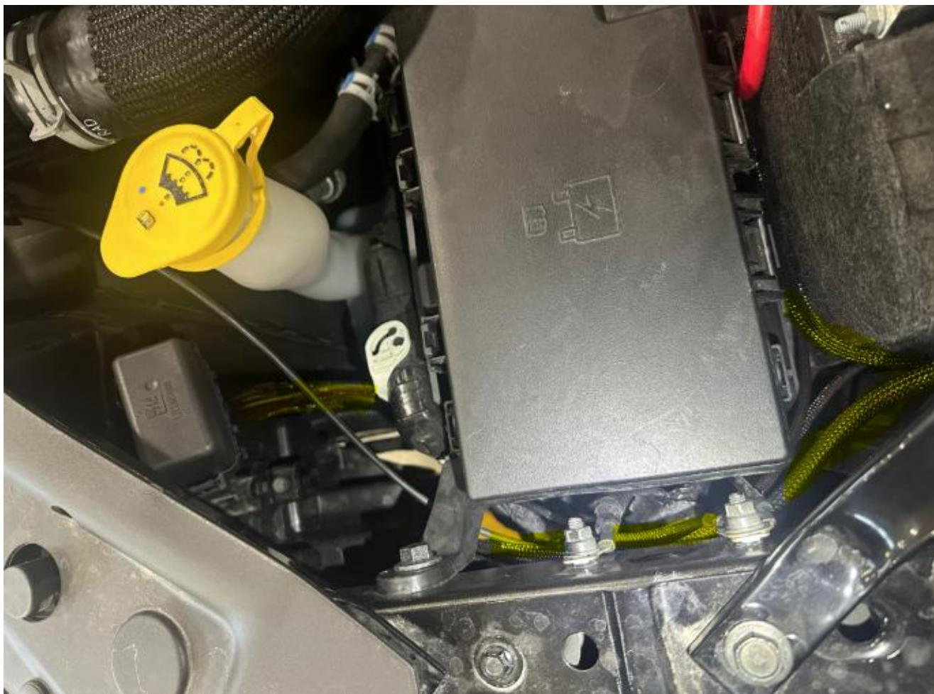
Route the single terminal between the battery and forward fuse box.
