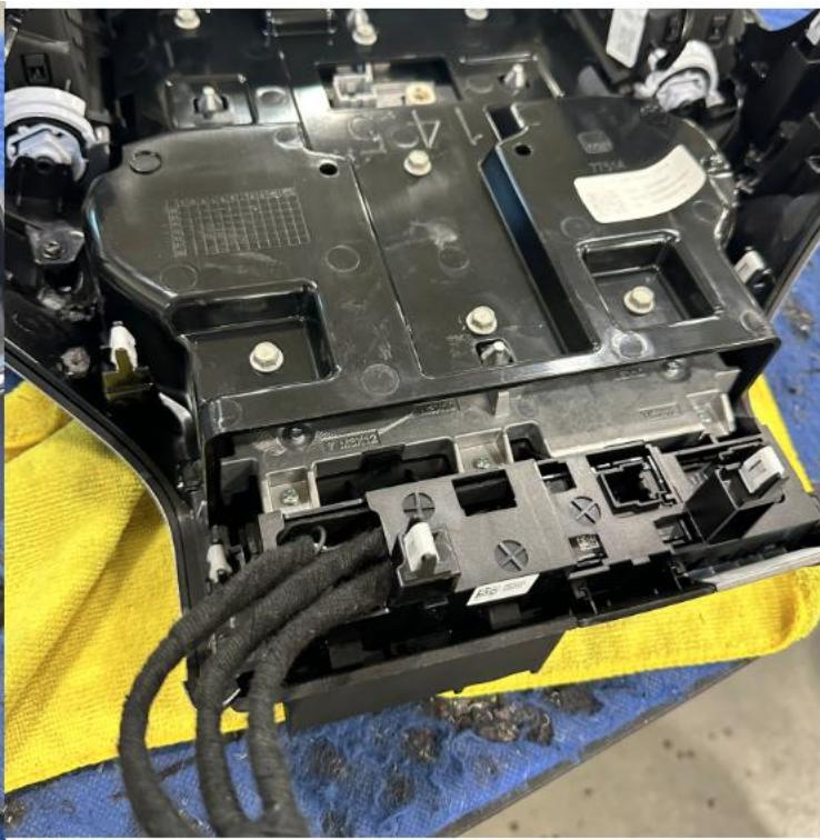
Snap the AEV switch bezel into the display.
