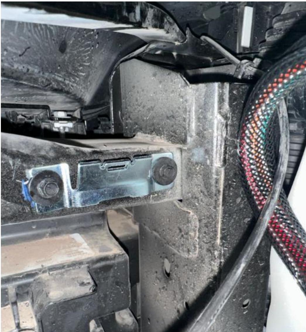
Remove the fuse box mounting bracket from the fuse box and secure with the provided screws.
