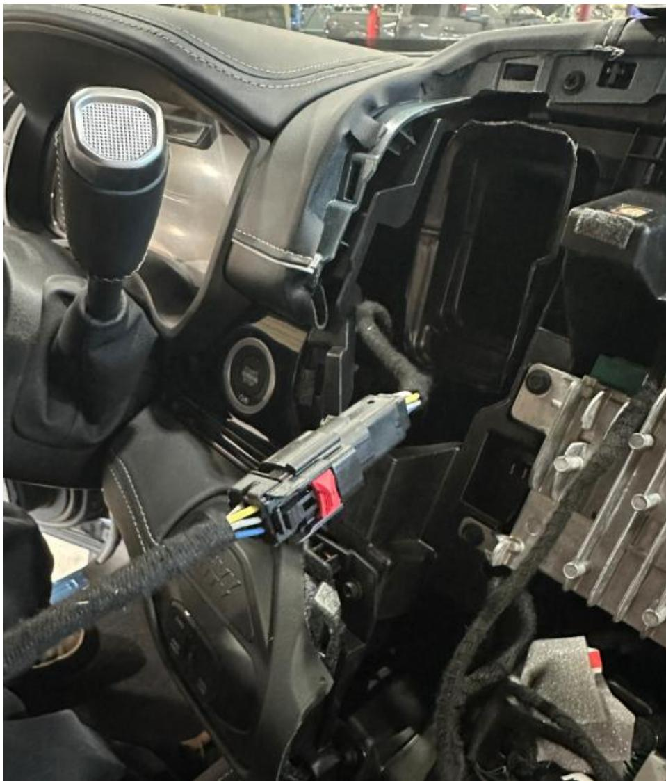
Plug the AEV switch harness into the fuse harness
