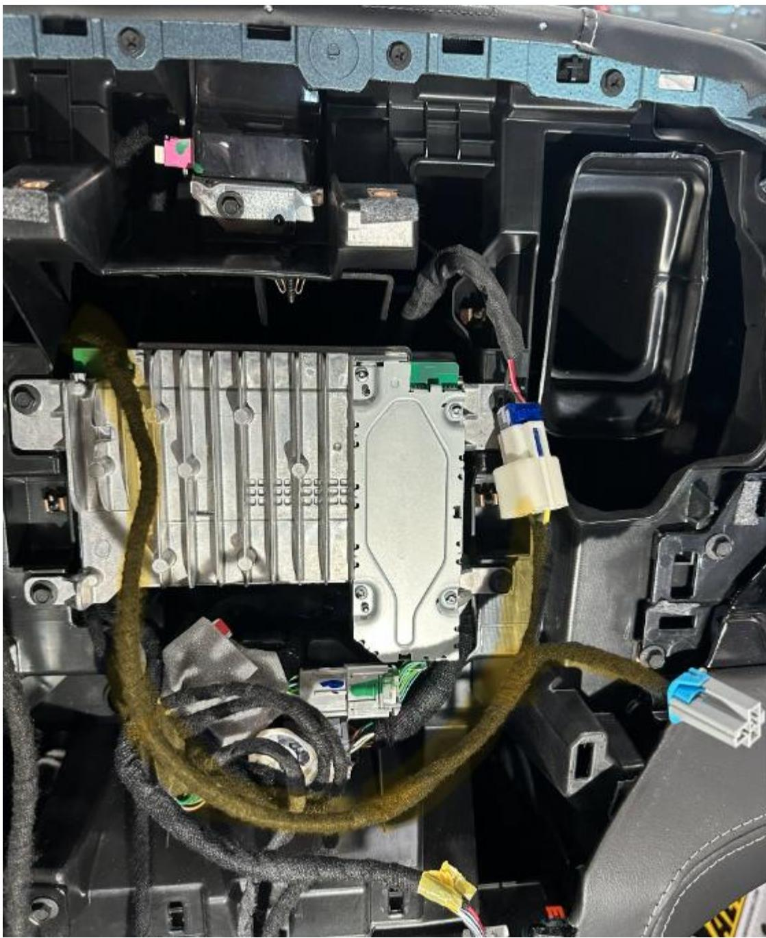
Connect the wide plug on the harness to the blue plug that originally went to the display
