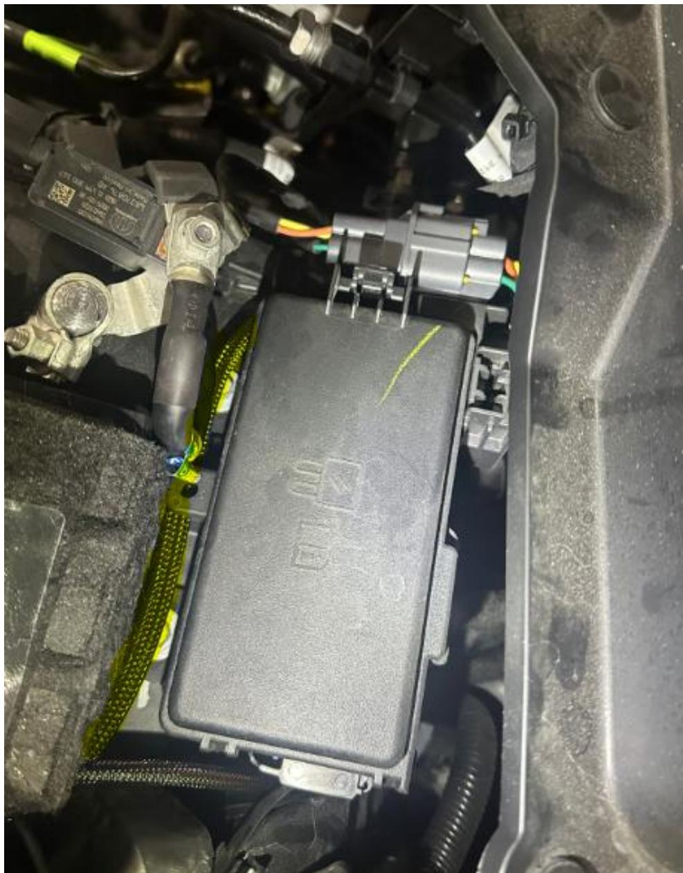
Begin routing the harness by passing between the fuse box and the battery
