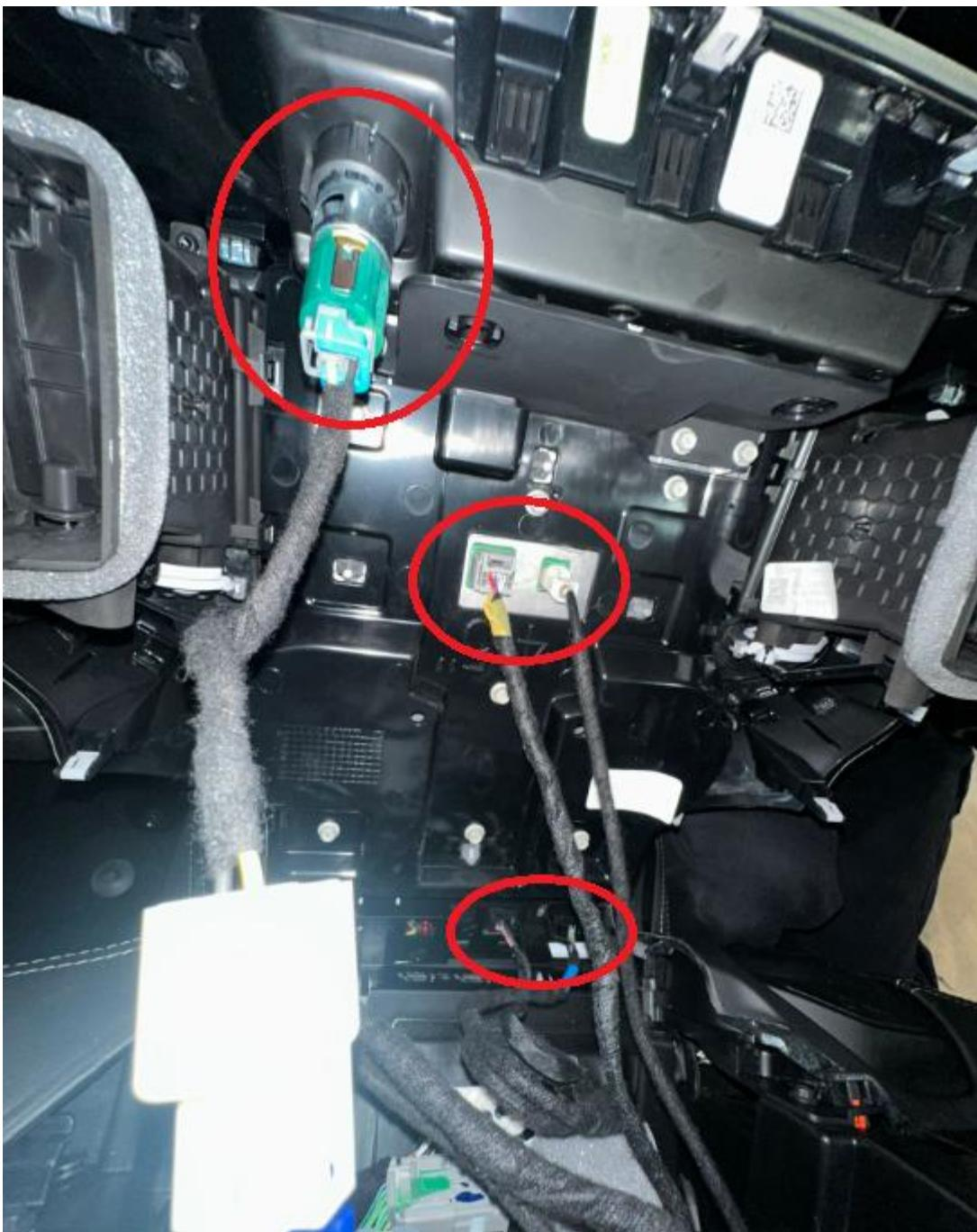
Once removed, the following harnesses need to be un-plugged from the back of the screen.
