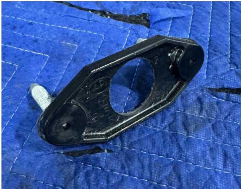
With the plate removed, drill a  $1 \frac{1}{2}$ " hole through the center. If your truck has a rubber seal between the plastic plate and steel, cut a hole large enough so that the harness can pass through.
