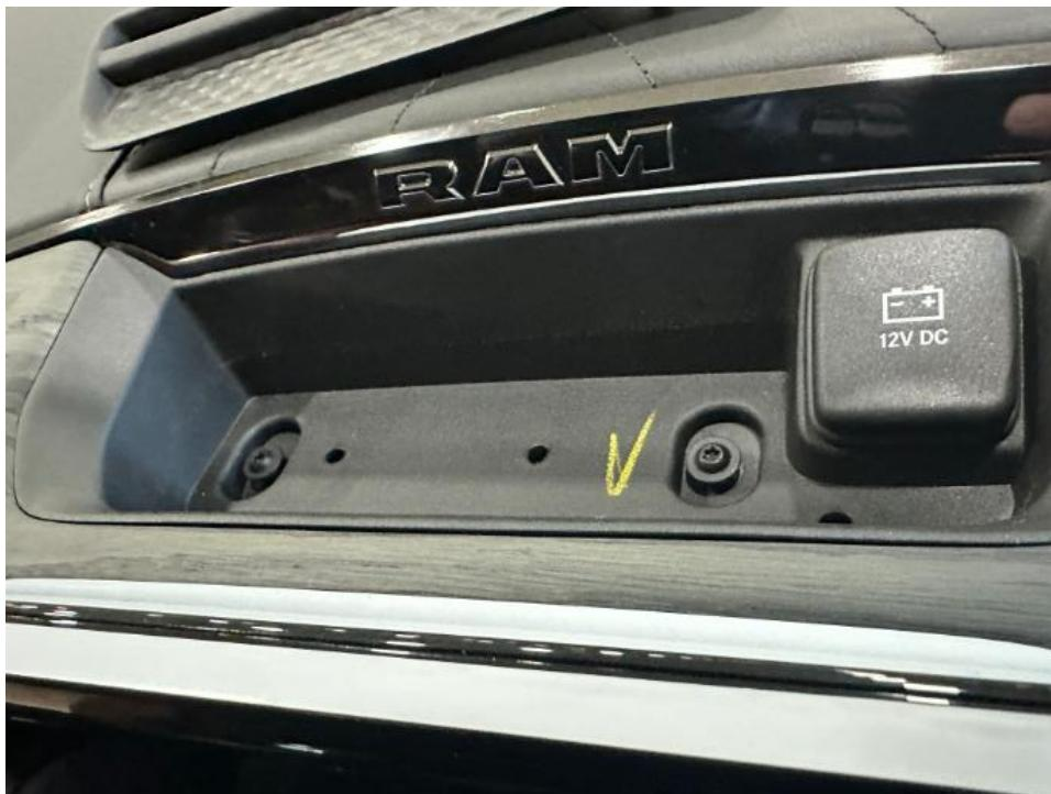
Once removed, you will have access to two T20 screws that can now be removed
