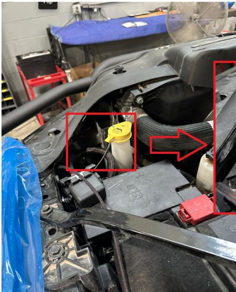
The fuse box is mounted to the support beam behind the headlight.
