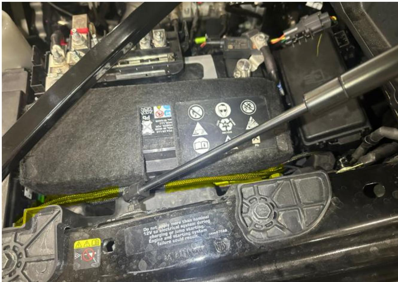
Continue routing alongside the battery, tucking the harness down along its side.
