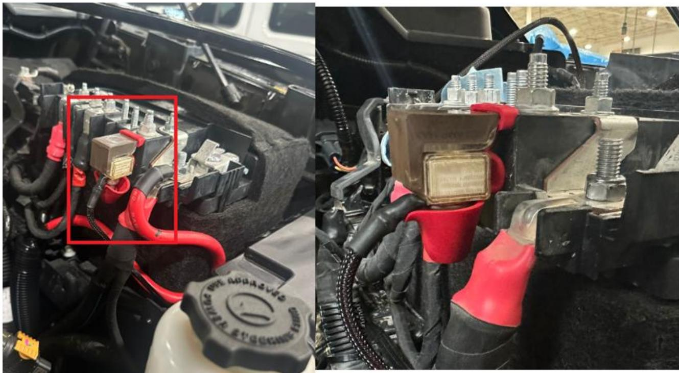
Using the provided fuse kit, take the power wire from the harness and secure it to the open terminal found on top of the battery on the driver's side.
