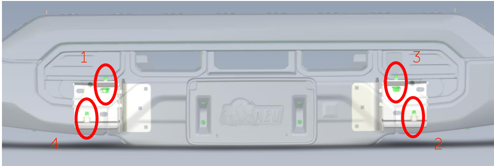
Figure 8 – M10 Torquing Sequence
